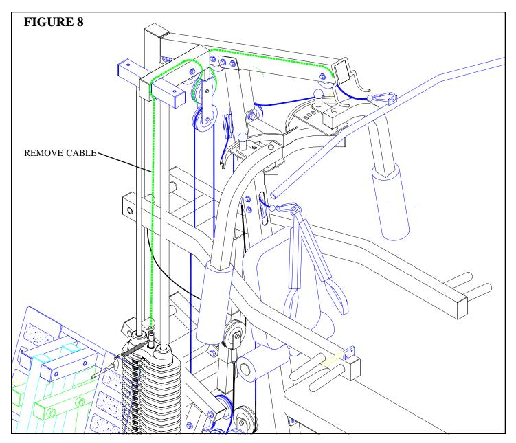
Remove the existing LAT CABLE using the following steps:
